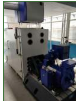
30 kW, 150kW , 220 kW E-Motor Test bed With Environmental Chamber
