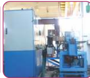
50KW Induction Billet Heater
